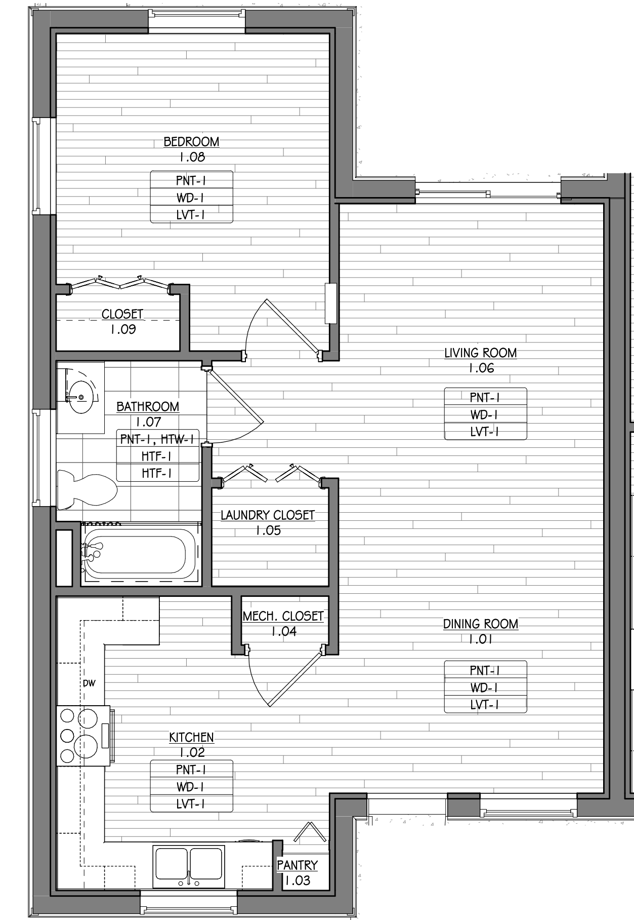
A1 FINISH PLAN - ONE BEDROOM UNIT SCALE: 1/4" = 1'-0"
